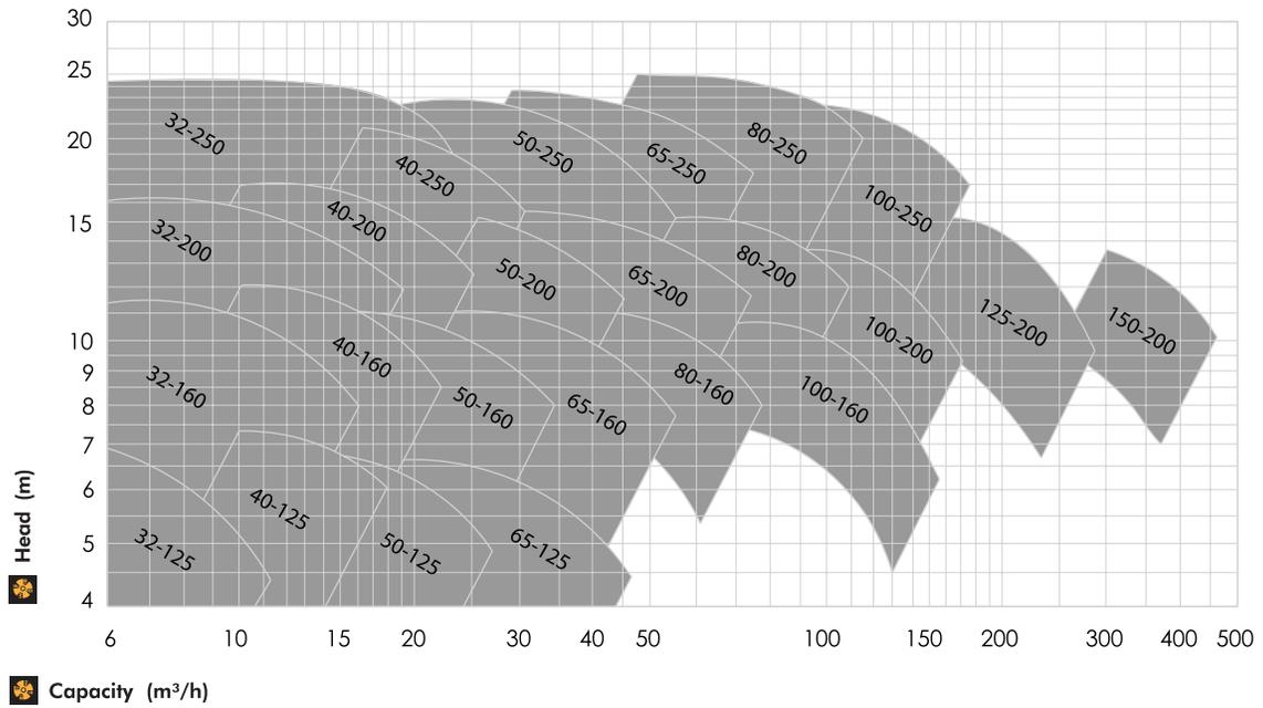
**2900 rpm / (d/d) (50 Hz)**
